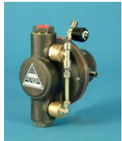
VP12-210S in cast iron with teflon-coated pump housing and quick-through valves. Can be supplied with diaphragms in various materials depending on what is to be pumped.
