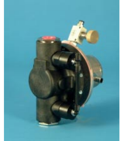
VP18S - in acetal plastic (POM) with bayonet locking of servo housing for rapid dismantling and equipped with quick-through valves. Diaphragms and O-rings available in various materials depending on what is to be pumped.
