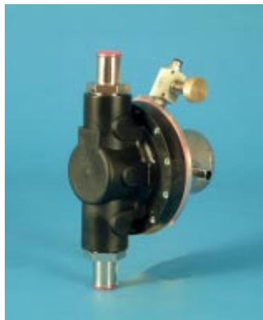
VP18 - in acetal plastic (POM) with bayonet locking of servo housing that allows rapid dismantling. Can be equipped with diaphragms and O-rings in various materials depending on what is to be pumped.
